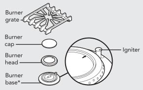
\* **Note:** When replacing burner head, arrow must be pointing towards back of range.
